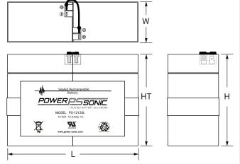
**L**: 8.45 (215) **W**: 2.75 (70) **H:** 5.75 (146) Tolerances are +/- 0.04 in. (+/- 1mm) and +/- 0.08 in. (+/- 2mm) for height dimensions. All data subject to change without notice.
